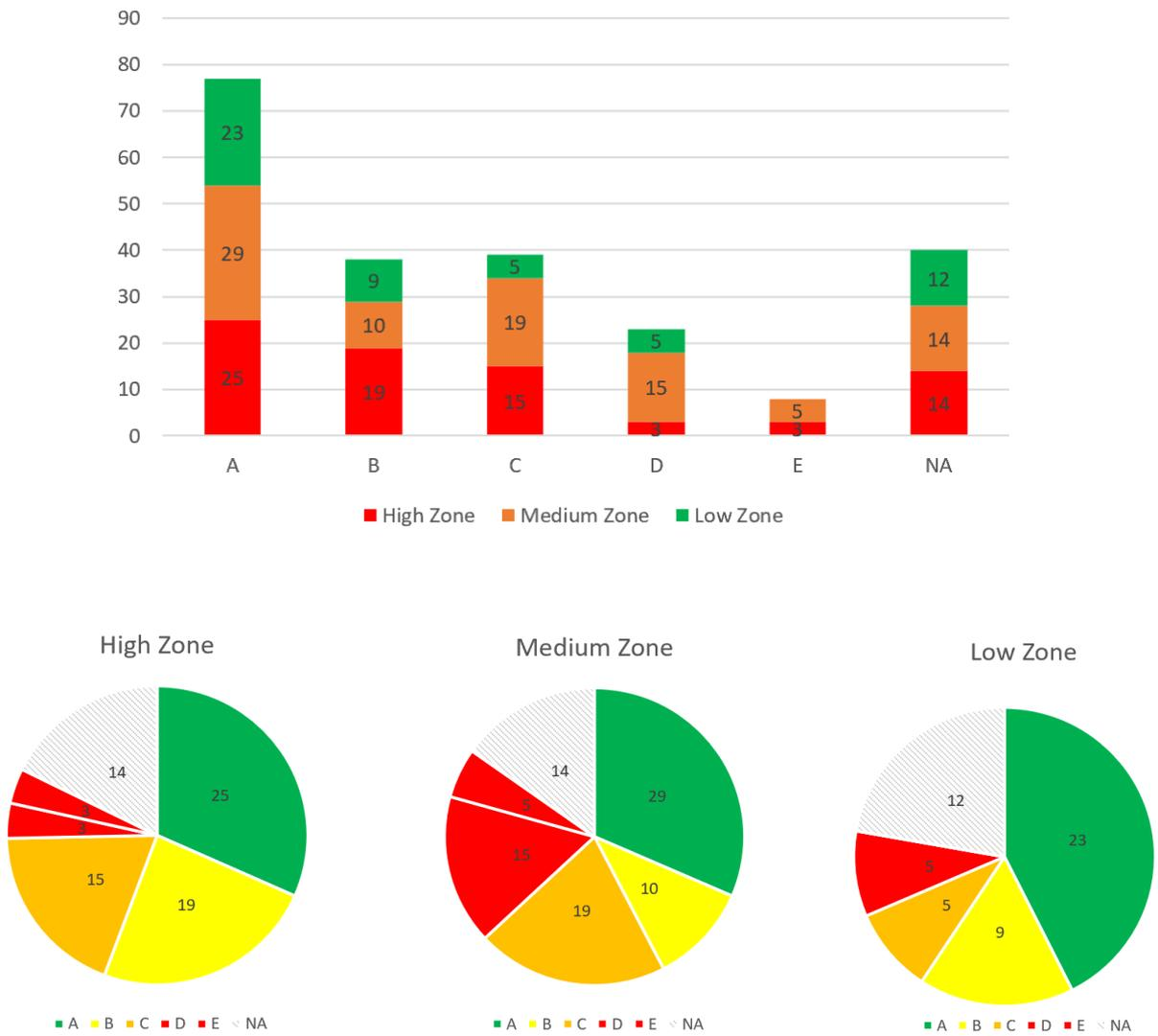
Figure 4.2: Seismic Ratings for IL4 Buildings
